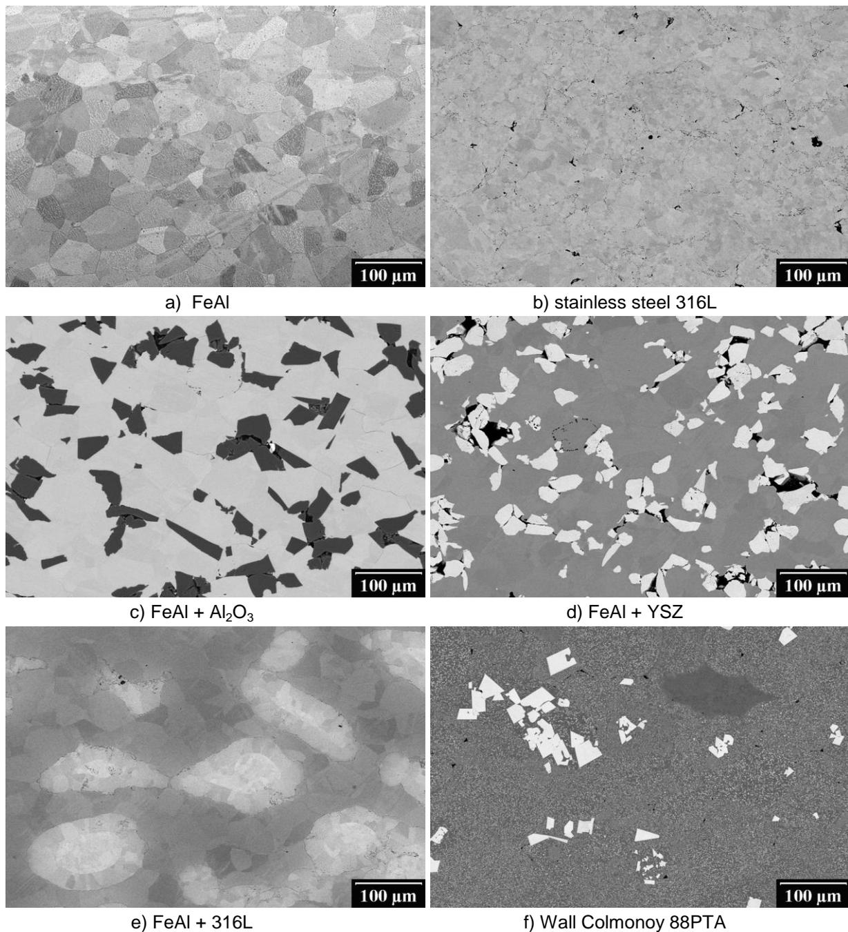
**Fig. 2** Microstructures of the sintered compacts
