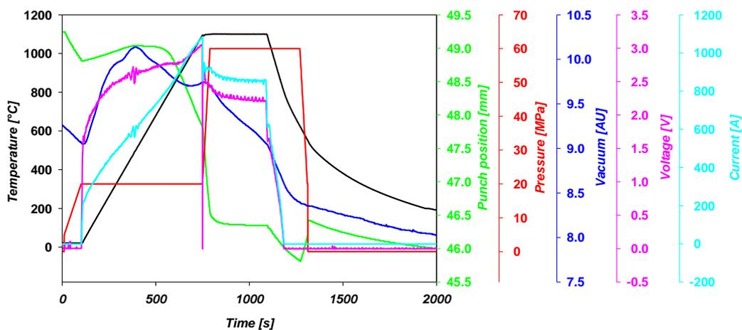
**Fig. 1** Record of sintering of FeAl + Al<sub>2</sub>O<sub>3</sub> sample
