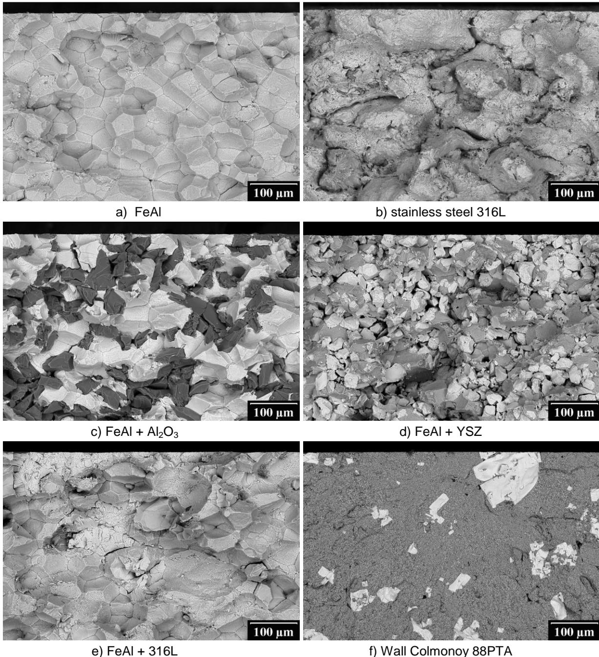
**Fig. 3** Fractographs of samples after 3-point bending test
